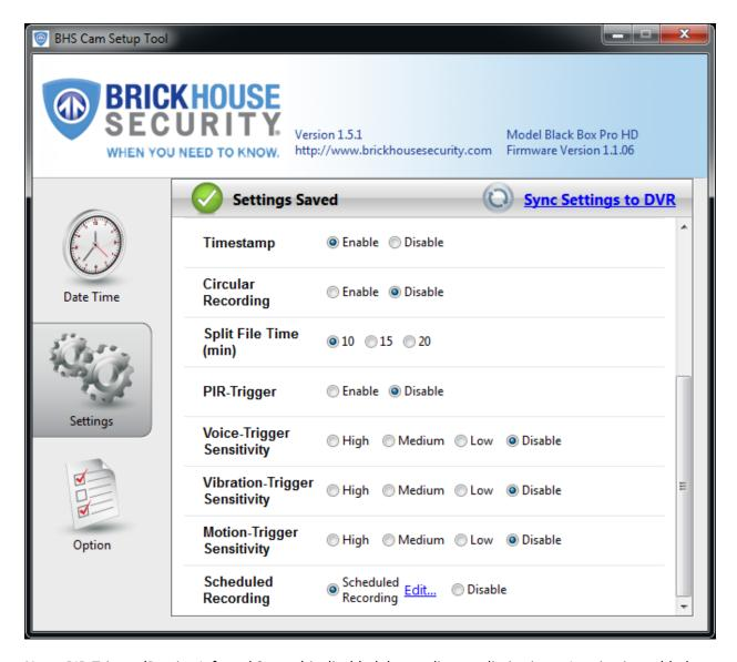
**Note:** PIR-Trigger (Passive Infrared Sensor) is disabled due to distance limitations. Leaving it enabled can decrease battery life.
