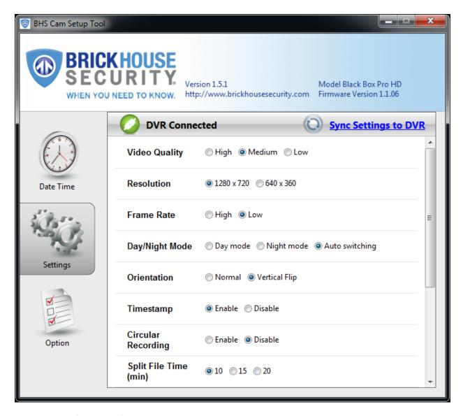
**Note:** Vertical flip allows for proper orientation, otherwise your videos will be up-side-down.
