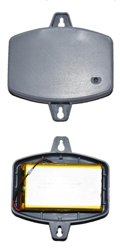
Place rear cover to front cover and press it one until flush with the front cover. Make sure to not pinch the camera wire or battery.
