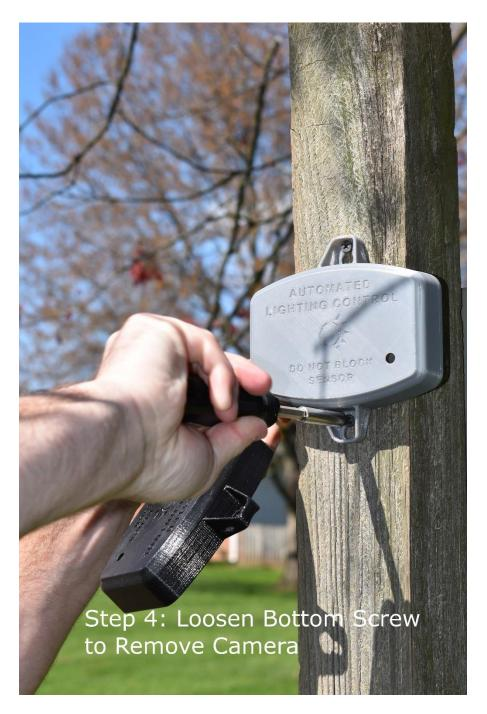
**Note:** Do not use power drill to tighten screws against the Dissembler. Over-tightening can damage the cover.
